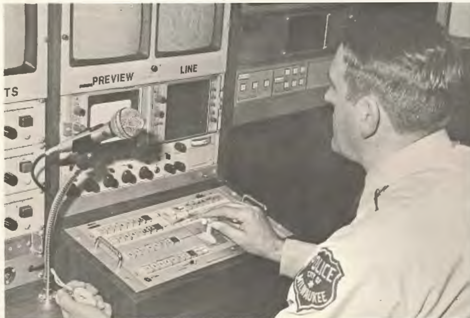
Master Television Console, Switcher, and Special Effects Generator
