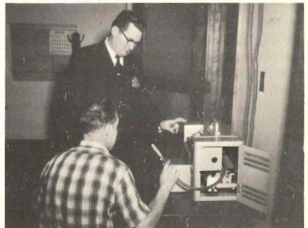
An 'Alcometer', the latest scientific device for determining the degree of intoxication, was placed in service in 1954.
